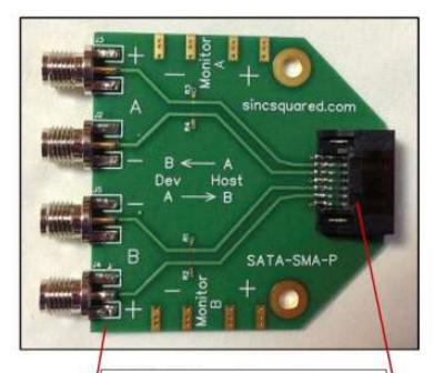
Standard configuration includes 4 SMA connectors. **Optional:** add 4 additional monitor SMA connectors (for 8 SMA connectors total).
