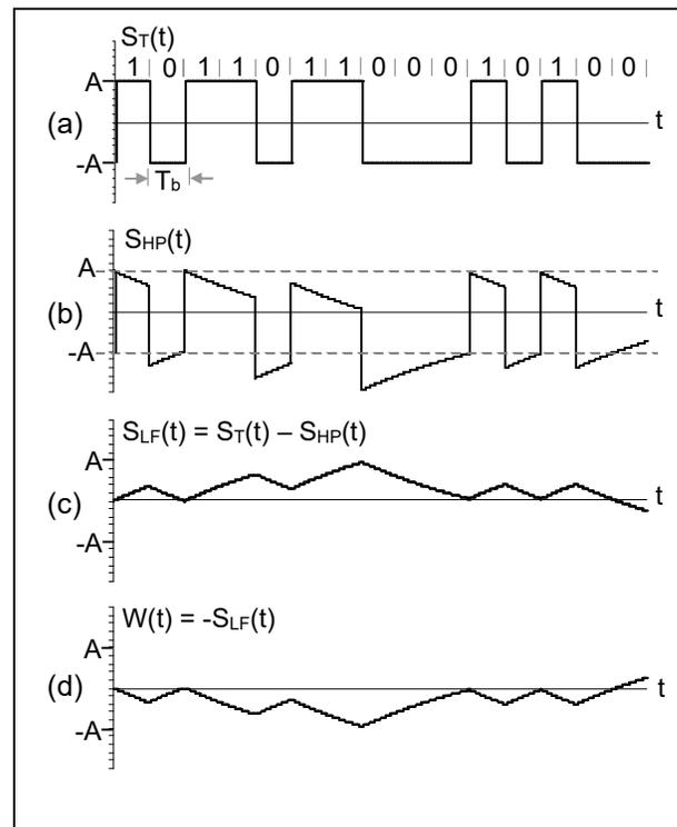
Figure 5. (a) Transmitted signal  $S_T(t)$ , (b) High-pass filtered signal  $S_{HP}(t)$ , (c) Filtered out low-frequency component of signal,  $S_{LF}(t) = S_T(t) - S_{HP}(t)$ , and (d) Baseline wander  $W(t) = -S_{LF}(t)$ .
